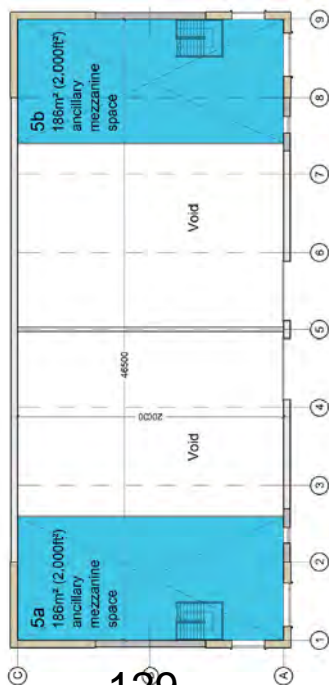
Unit 5 - Mezzanine Floor Plan
